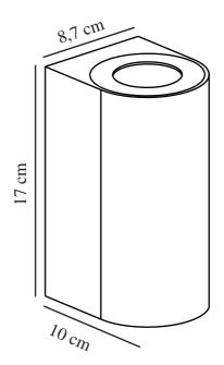
Voltage (V): 230 Volt IP degree: IP44 Maximum bulb wattage (W): 28 Class (Class 1, Class 2, Class 3): Class 1 (Earth contact) Socket type: GU10
