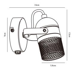
Voltage (V): 230 Volt IP degree if the fixture includes two types of IP degree: IP20 Maximum compatible bulb wattage (W): 35W Class (Class I, Class II, Class III): Class 2 (Double isolated) Lampholder type (eg, E27/E14, etc): G9
