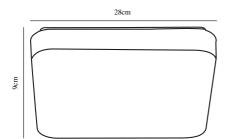
Voltage (V): 230 Volt IP degree if the fixture includes two types of IP degree: IP20 Class (Class I, Class II, Class III): Class 1 (Earth contact) Lampholder type (eg, E27/E14, etc): LED Module Parallel connection possible?: False
