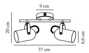
Voltage (V): 230 Volt IP degree: IP20 Maximum bulb wattage (W): 2X40W
