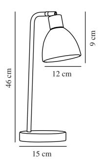
Voltage (V): 220-240 Volt IP degree: IP20
