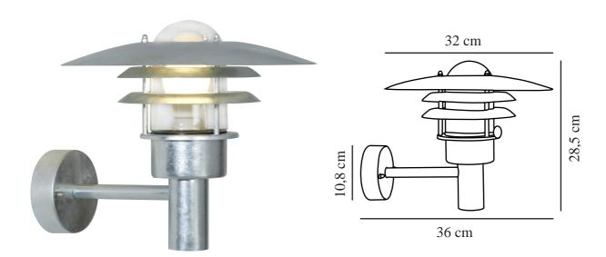
Voltage (V): 230 Volt IP degree: IP44 Maximum bulb wattage (W): 60 Class (Class 1, Class 2, Class 3): Class 2 (Double isolated) Socket type: E27 Parallel connection: True
