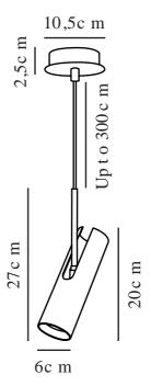
Voltage (V): 220-240 Volt IP degree: IP20
