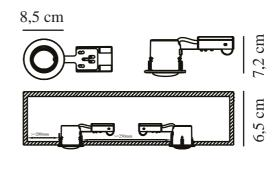
Voltage (V): 230 Volt IP degree: IP23 Maximum bulb wattage (W): 8 Class (Class 1, Class 2, Class 3): Class 2 (Double isolated) Socket type: GU10 Parallel connection: True
