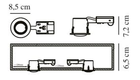
Voltage (V): 220-240 Volt IP degree: IP23 Maximum bulb wattage (W): 8W LED Class (Class 1, Class 2, Class 3): Class 2 (Double isolated) Socket type: GU10 Parallel connection: True
