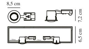
Voltage (V): 230 Volt IP degree: IP23 Maximum bulb wattage (W): 8 Class (Class 1, Class 2, Class 3): Class 2 (Double isolated) Socket type: GU10 Parallel connection: True
