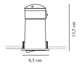
Voltage (V): 230 Volt IP degree: IP23 Maximum bulb wattage (W): 8 Class (Class 1, Class 2, Class 3): Class 2 (Double isolated) Socket type: GU10 Parallel connection: True
