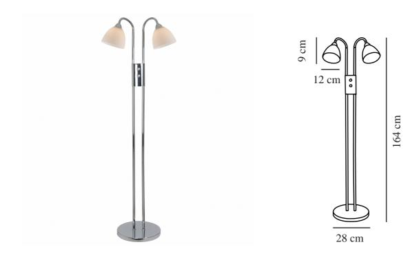
Voltage (V): 230 Volt IP degree: IP20 Maximum bulb wattage (W): 2X40W Class (Class 1, Class 2, Class 3): Class 2 (Double isolated) Socket type: E14 Dimmerable: Yes with compatible bulb Switch placement: On the fixture
