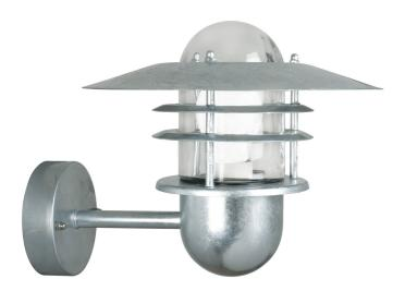
Voltage (V): 230 Volt IP degree: IP54 Maximum bulb wattage (W): 60 Class (Class 1, Class 2, Class 3): Class 2 (Double isolated) Socket type: E27 Parallel connection: True
