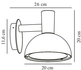
Voltage (V): 230 Volt IP degree: IP54 Maximum bulb wattage (W): 20 Class (Class 1, Class 2, Class 3): Class 1 (Earth contact) Socket type: E27 Parallel connection: True
