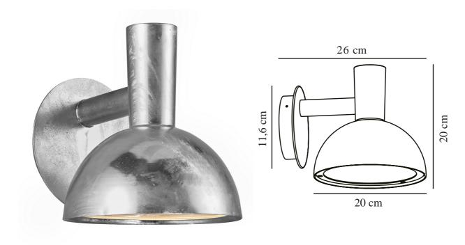
Voltage (V): 230 Volt IP degree: IP54 Maximum bulb wattage (W): 20 Class (Class 1, Class 2, Class 3): Class 1 (Earth contact) Socket type: E27 Parallel connection: True
