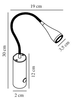
Voltage (V): 230 Volt IP degree: IP20 Class (Class 1, Class 2, Class 3): Class 3 (12V) Socket type: LED Module Switch placement: On the fixture
