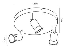
Voltage (V): 230 Volt IP degree if the fixture includes two types of IP degree: IP20 Maximum compatible bulb wattage (W): 3X3W Class (Class I, Class II, Class III): Class 1 (Earth contact) Lampholder type (eg, E27/E14, etc): GU10
