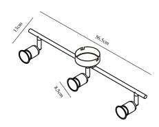
Voltage (V): 230 Volt IP degree if the fixture includes two types of IP degree: IP20 Maximum compatible bulb wattage (W): 3X35W Class (Class I, Class II, Class III): Class 1 (Earth contact) Lampholder type (eg, E27/E14, etc): GU10
