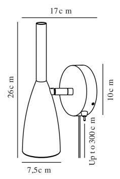
Voltage (V): 230 Volt IP degree: IP20
