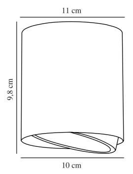
Voltage (V): 230 Volt IP degree: IP44 Maximum bulb wattage (W): 6W LED Class (Class 1, Class 2, Class 3): Class 2 (Double isolated) Socket type: GU10
