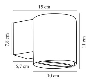
Voltage (V): 230 Volt IP degree: IP44 Maximum bulb wattage (W): 8W LED Class (Class 1, Class 2, Class 3): Class 2 (Double isolated)
