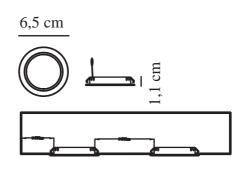
Voltage (V): 12 Volt IP degree: IP20/23 Class (Class 1, Class 2, Class 3): Class 3 (12V) Socket type: LED – Nonreplaceable light source Switch placement: On the cable Parallel connection: False
