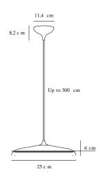
Voltage (V): 230 Volt IP degree if the fixture includes two types of IP degree: IP20 Class (Class I, Class II, Class III): Class 2 (Double isolated) Lampholder type (eg, E27/E14, etc): LED Module Dimmerable: True
