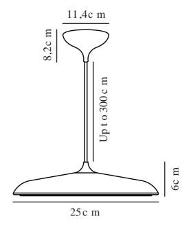
Voltage (V): 230 Volt IP degree: IP20 Class (Class 1, Class 2, Class 3): Class 2 (Double isolated) Socket type: LED Module Dimmerable: True
