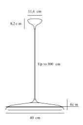
Voltage (V): 230 Volt IP degree if the fixture includes two types of IP degree: IP20 Class (Class I, Class II): Class 2 (Double isolated) Lampholder type (eg, E27/E14, etc): LED Module Dimmerable: True
