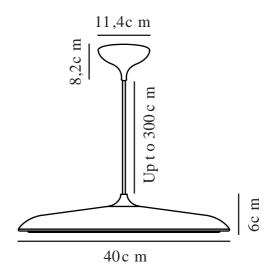
Voltage (V): 230 Volt IP degree: IP20 Class (Class 1, Class 2, Class 3): Class 2 (Double isolated) Socket type: LED Module Dimmerable: True
