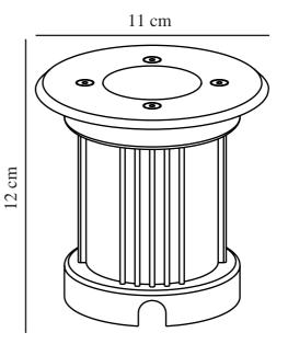
Voltage (V): 230 Volt IP degree: IP65 Maximum bulb wattage (W): 35W Class (Class 1, Class 2, Class 3): Class 1 (Earth contact) Socket type: GU10 Parallel connection: False
