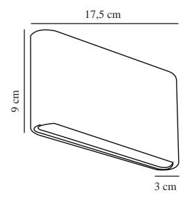
Voltage (V): 220-240 Volt IP degree: IP54 Class (Class 1, Class 2, Class 3): Class 1 (Earth contact) Socket type: LED – Nonreplaceable light source Parallel connection: False
