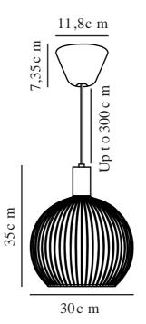
Voltage (V): 230 Volt IP degree: IP20
