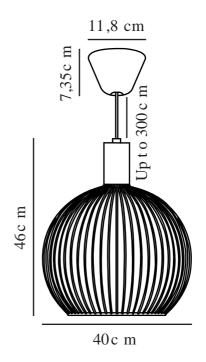
Voltage (V): 230 Volt IP degree: IP20 Maximum bulb wattage (W): 60 Class (Class 1, Class 2, Class 3): Class 2 (Double isolated) Socket type: E27 Dimmerable: Yes with compatible
