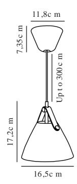
Voltage (V): 220-240 Volt IP degree: IP20 Maximum bulb wattage (W): 40 Class (Class 1, Class 2, Class 3): Class 2 (Double isolated) Socket type: GU10 Dimmerable: Yes with compatible bulb Parallel connection: False
