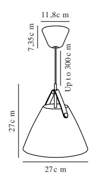
Voltage (V): 220-240 Volt IP degree: IP20 Maximum bulb wattage (W): 40 Class (Class 1, Class 2, Class 3): Class 2 (Double isolated) Socket type: E27 Dimmerable: Yes with compatible bulb Parallel connection: False
