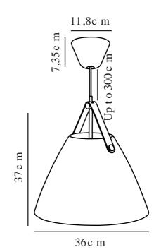
Voltage (V): 220-240 Volt IP degree: IP20 Maximum bulb wattage (W): 40 Class (Class 1, Class 2, Class 3): Class 2 (Double isolated) Socket type: E27 Dimmerable: Yes with compatible bulb Parallel connection: False
