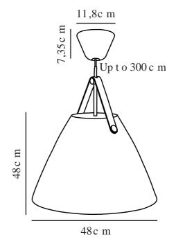
IP degree: IP20 Maximum bulb wattage (W): 40 Class (Class 1, Class 2, Class 3): Class 2 (Double isolated) Socket type: E27
