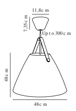
Voltage (V): 220-240 Volt IP degree: IP20 Maximum bulb wattage (W): 40 Class (Class 1, Class 2, Class 3): Class 2 (Double isolated) Socket type: E27 Dimmerable: Yes with compatible bulb Parallel connection: False
