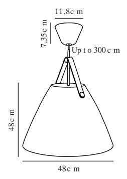
IP degree: IP20 Maximum bulb wattage (W): 40W Class (Class 1, Class 2, Class 3): Class 2 (Double isolated) Socket type: E27
