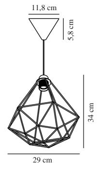
Voltage (V): 230 Volt IP degree: IP20
