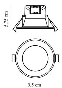
Voltage (V): 230 Volt IP degree: IP20 Class (Class 1, Class 2, Class 3): Class 2 (Double isolated) Socket type: LED – Nonreplaceable light source Dimmerable: True Parallel connection: True
