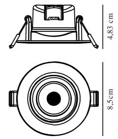
Voltage (V): 220-240 Volt IP degree: IP23 Class (Class 1, Class 2, Class 3): Class 2 (Double isolated) Socket type: LED – Nonreplaceable light source Dimmerable: True Parallel connection: True
