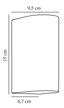
Voltage (V): 230 Volt IP degree: IP44 Class (Class 1, Class 2, Class 3): Class 1 (Earth contact) Socket type: LED – Nonreplaceable light source Parallel connection: True
