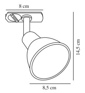
Voltage (V): 230 Volt IP degree: IP20 Maximum bulb wattage (W): 35W Class (Class 1, Class 2, Class 3): Class 1 (Earth contact) Socket type: GU10
