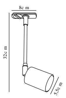
Voltage (V): 220-240 Volt IP degree: IP20 Maximum bulb wattage (W): 35 Class (Class 1, Class 2, Class 3): Class 2 (Double isolated) Socket type: GU10
