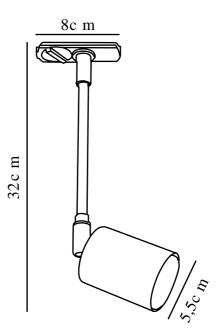
Voltage (V): 220-240 Volt IP degree: IP20 Maximum bulb wattage (W): 35 Class (Class 1, Class 2, Class 3): Class 2 (Double isolated) Socket type: GU10 Parallel connection: False
