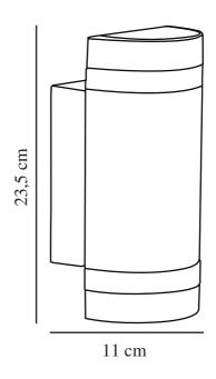
Voltage (V): 230 Volt IP degree: IP44 Maximum bulb wattage (W): 35 Class (Class 1, Class 2, Class 3): Class 1 (Earth contact) Socket type: GU10 Parallel connection: True
