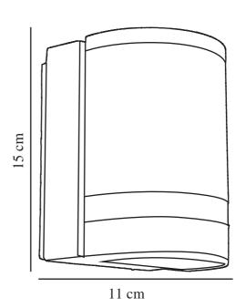
Voltage (V): 230 Volt IP degree: IP44 Maximum bulb wattage (W): 35W Class (Class 1, Class 2, Class 3): Class 1 (Earth contact) Socket type: GU10 Parallel connection: True
